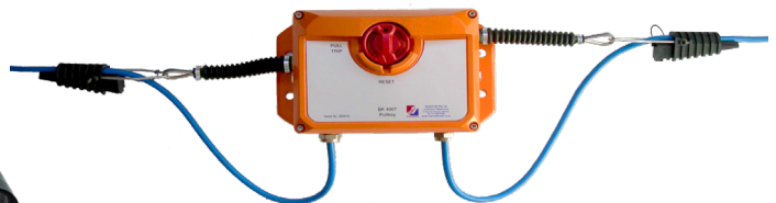
Control Pull Cable secured with Wedge Clamps
