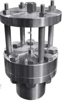
Rupture Pin Technology's **Model H** is best in Methanol and Chemical Injection Systems and is available for pressure set points up to 20,000 PSI. The product is an angle valve that holds a bubble-tight, closed position until the pressure reaches an exact point, at which time the valve will open within milliseconds creating minimal exposure of the flow to the piston. The Model H is unaffected by pulsating pressure or changing ambient temperate at the pin.
